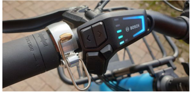
Replacement bell and the controller switchgear
