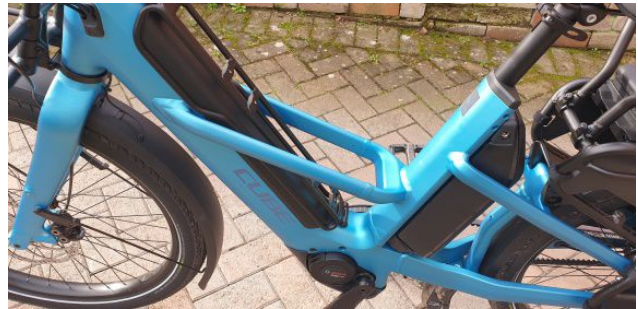
Frame storage and the Bosch battery and motor
