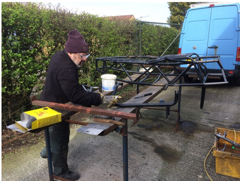
April 2020 John and Dan paint strip first build's powder coat off body frame. Filthy long job!! Necessary due to frame modifications.
