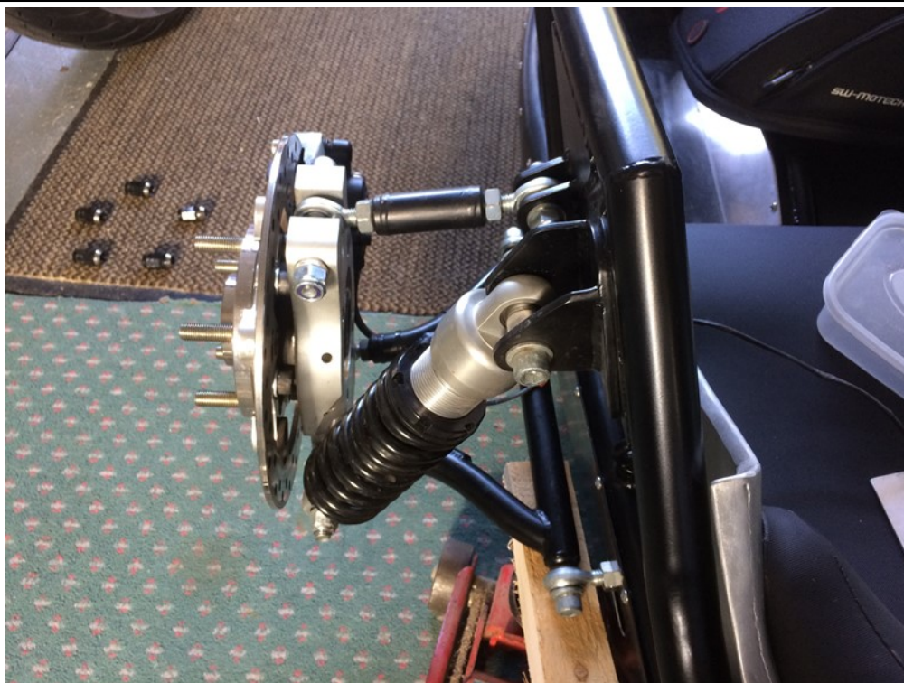
May 2020 Ultra neat Sidecar suspension re-engineered by Paul and Ricky. Still half wishbone, yet now truly compact! Wheel much closer to body.
