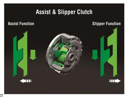
and grip before the correct gear is selected and speed matching between engine and transmission is once again achieved.
