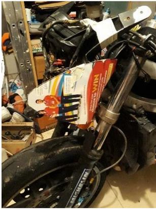
that not only would do the job of holding the light but also the indicators. One cornflake packet later and I had a template. Another trip to Avery Knight and Bowlers' scrap bin and I had a 300mm by 150mm sheet of lightweight aluminium, this I was able to cut with scissors and then form to give me a rigidish profile of the final job. Next my lovely sheet of stainless steel. The same sheet that I had used to make the fishplates for
