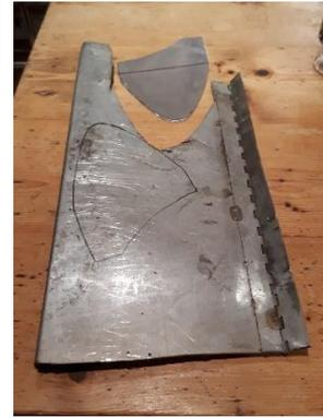
the sub-frame, the same sheet that I pulled from a hedge on the A46 on the way up to Dyrham Park. I won't pretend that cutting it was easy work, it wasn't but gently, gently with the jig saw and I had my plates. These I polished using odd bits of wet and dry and paraffin starting at around 300 grit and finishing with 1200 grit and metal paste.
